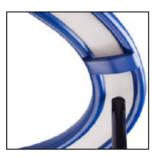
Curves can be covered without creasing if the profile is heated slightly more. The profile is stretched at the outer radius and compressed at the inner radius. It is necessary to ensure that the lower retaining section is in contact with the steel bar across its entire surface. Retaining bars (cut from the profile) can be welded onto the underside of the curves to ensure that the profile does not lift off.
