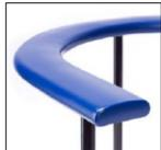
REHAU provides no guarantee for radii smaller than this. Once the fitted handrail has cooled, the ends are cut neatly leaving an extra 2 to 5 cm (depending on the profile length) to compensate for possible profile shrinkage. It is advisable to wait a few days before finishing this work.
